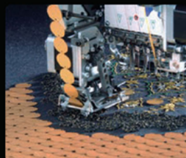
Sequin Device IV Embroidering various sequins: small-diameter sequins, large-diameter sequins, irregular-shaped sequins and eccentric sequins
