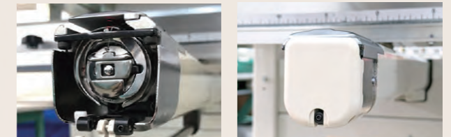
During bobbin replacement (Rotary hook cover open)
