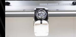
New thread trimming device eliminates the picker
